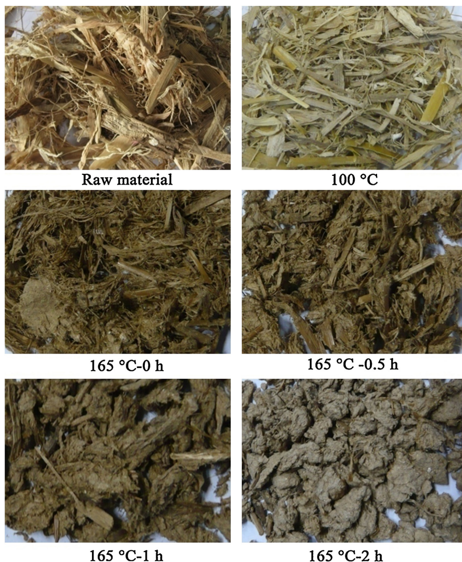
Fig. 1. The photographs of corn stalk and pulp in different cooking stages.
